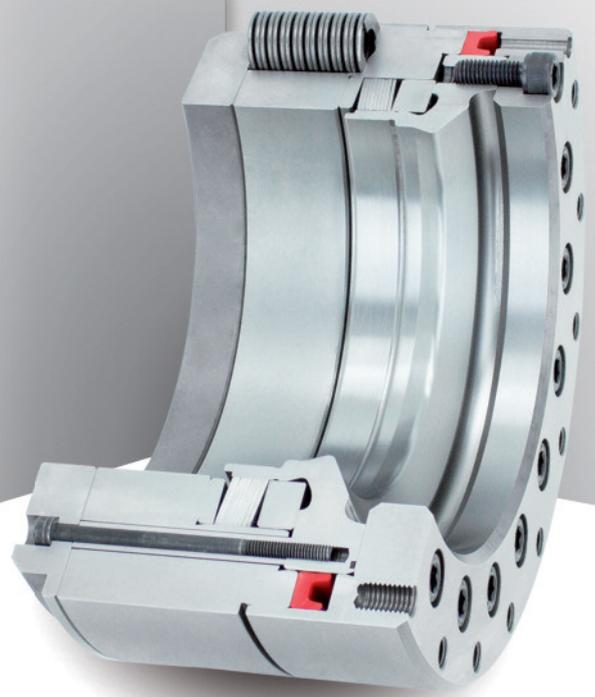
ment. This purely mechanical action ensures a fully anti-twist, all round clamping of the kingpin of the positioning axis. The clamping is quickly released by applying 115 bar of hydraulic pressure to the clamping coupling. This immediately frees the positioning axis of the rotary/swivel table again for the approach into the next angle setting. The new high-precision solution from RINGSPANN thus also supports quick changes between different angle settings of a machining process.
